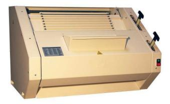
The vertical moulder is designed to laminate and to mould some pieces of dough which are intended to the making of baguettes, breads and small breads, in a little space.
